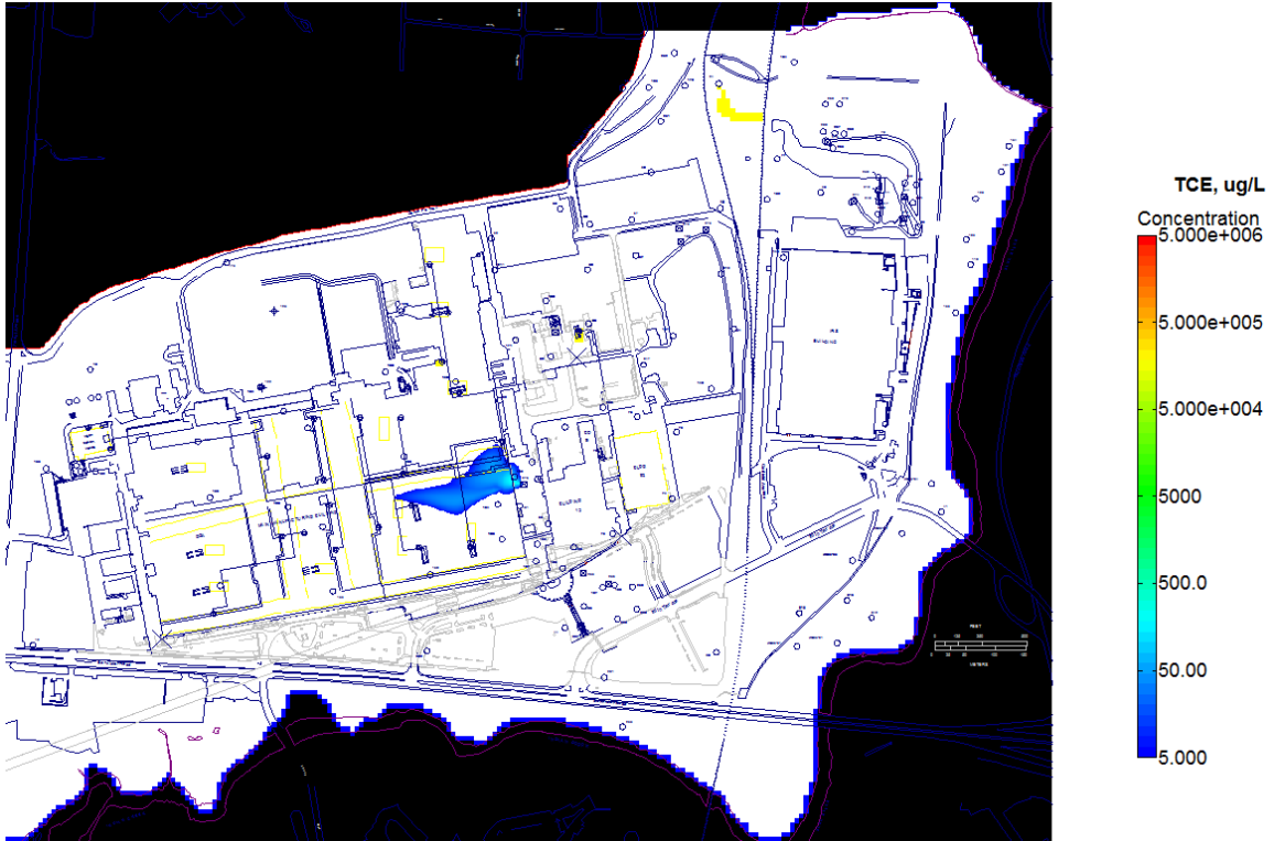
Current Conditions: TCE, Year 131, 131 year after source remediation
