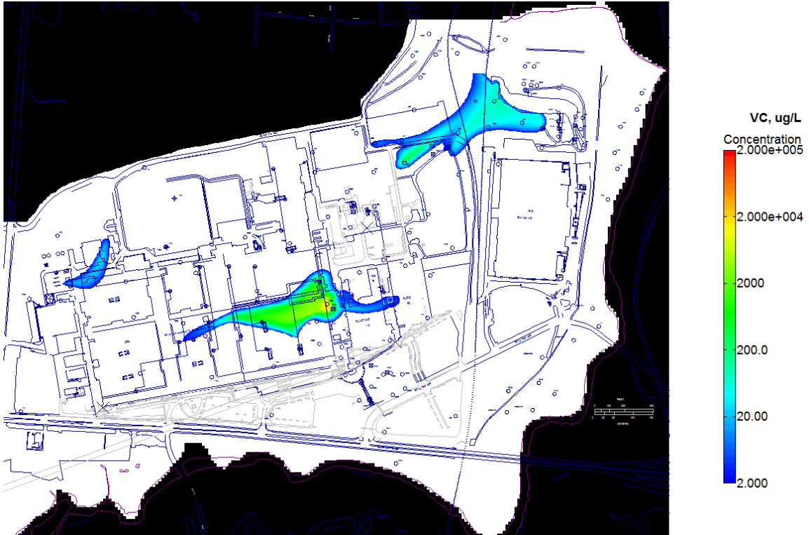
Current Conditions: VC, Years 1 through 250, constant source Current Conditions, No Source Reduction
