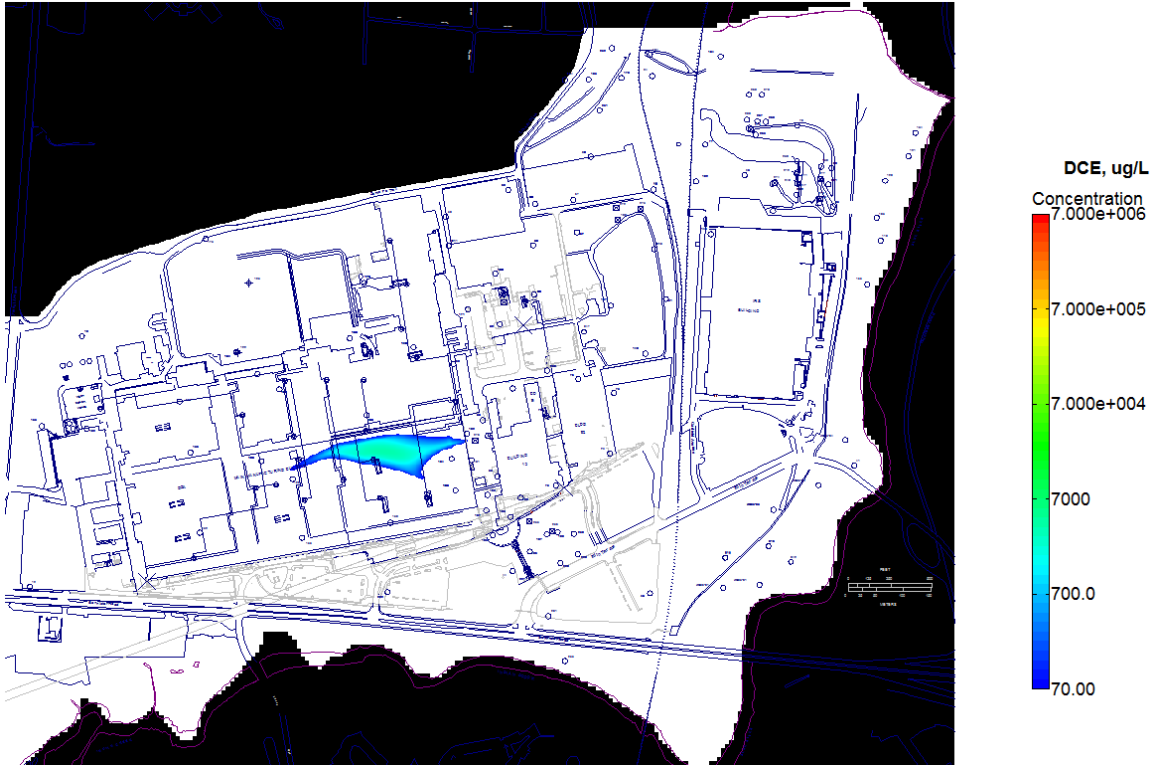
Current Conditions: DCE, Year 290, 40 years after complete source dilution
