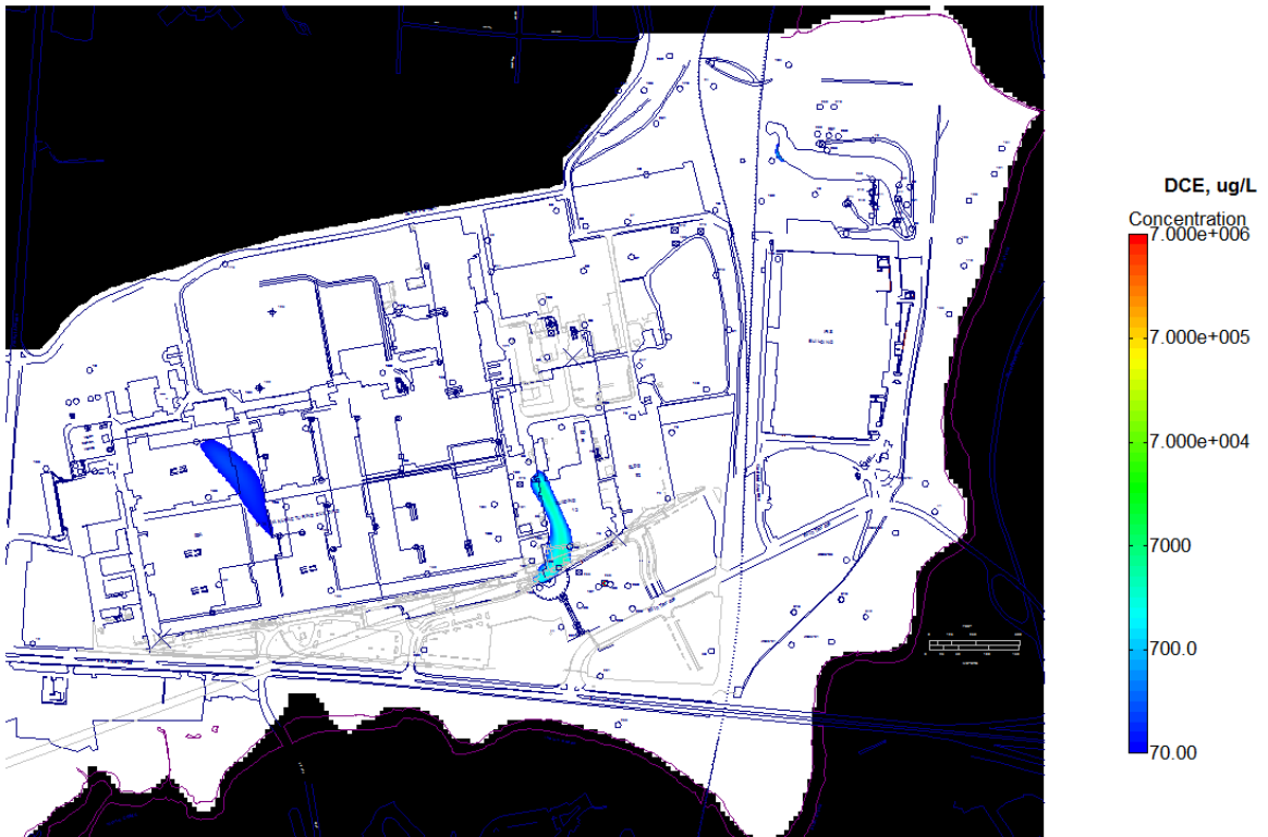
Future Conditions: DCE, Year 260, 10 years after complete source dilution Future Conditions, No Source Reduction
