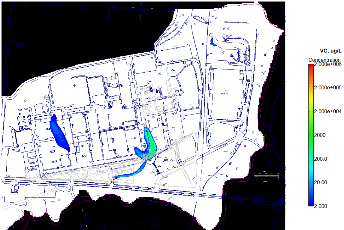
Future Conditions: VC, Year 17, 17 years after source remediation Future Conditions, 0% Source Concentration Reduction, 95% Source Duration Reduction
