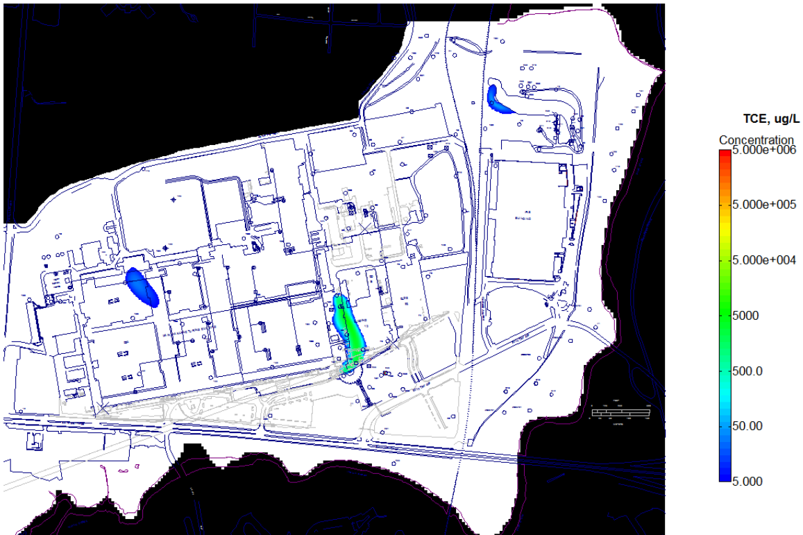
Future Conditions: TCE, Year 254, 4 years after complete source dilution Future Conditions, No Source Reduction
