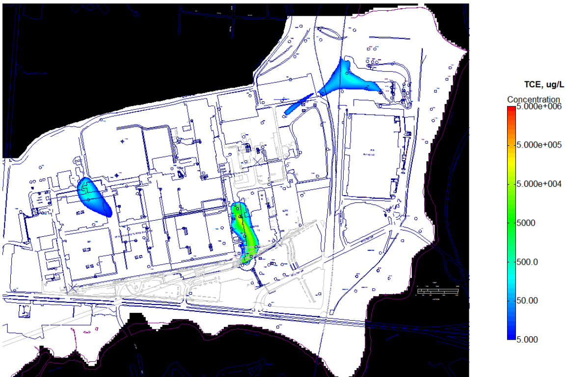
Future Conditions: TCE, Year 65, 2 years after complete source dilution Future Conditions, 0% Source Concentration Reduction, 75% Source Duration Reduction
