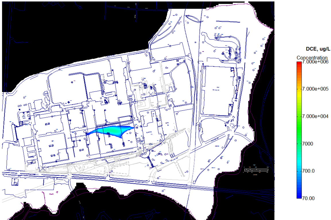
Current Conditions: DCE, Year 277, 277 years after source remediation
