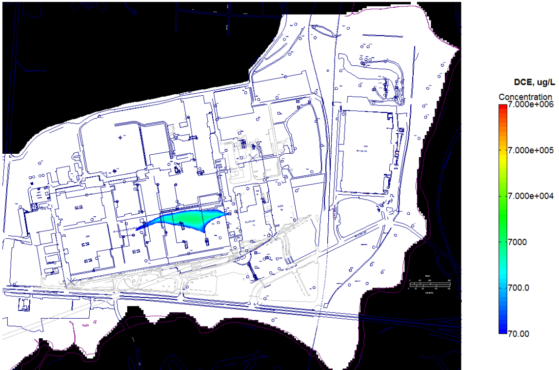
Current Conditions: DCE, Year 280, 30 years after complete source dilution
