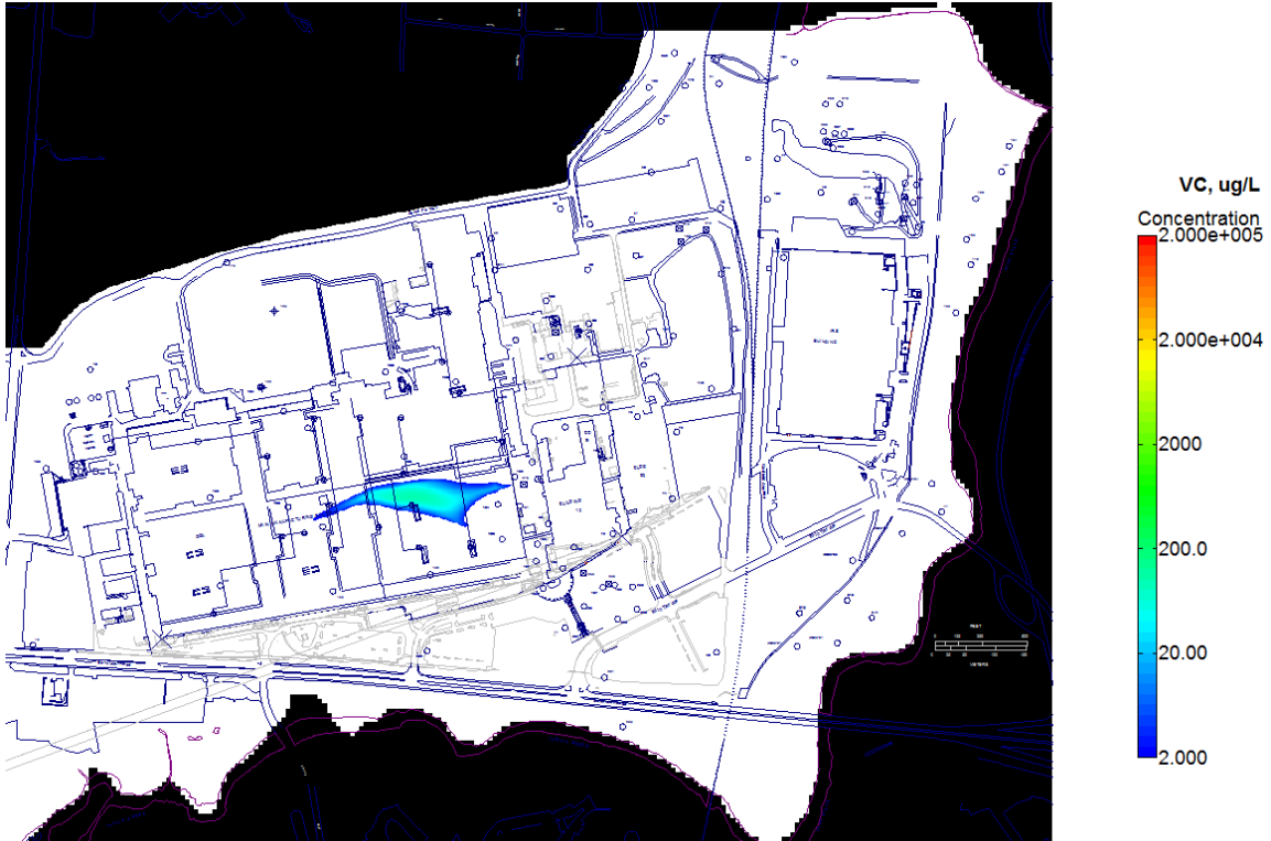
Current Conditions: VC, Year 300, 50 years after complete source dilution
