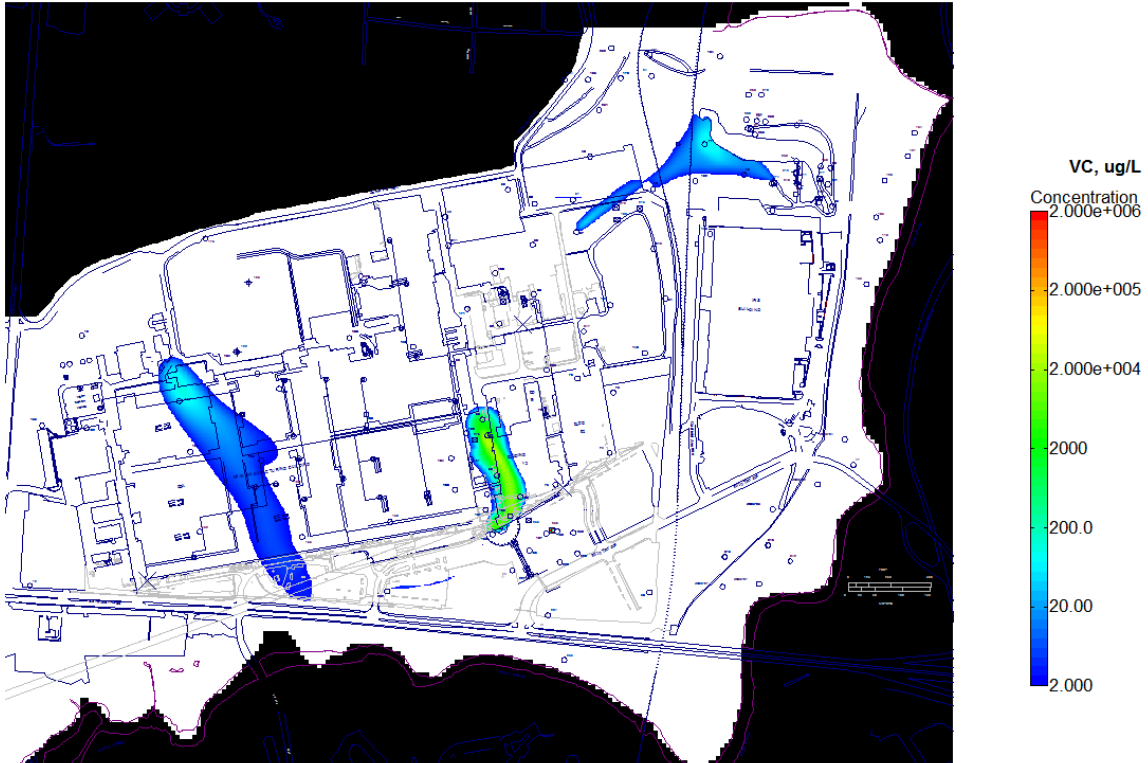
Future Conditions: VC, Year 252, 2 years after complete source dilution Future Conditions, No Source Reduction
