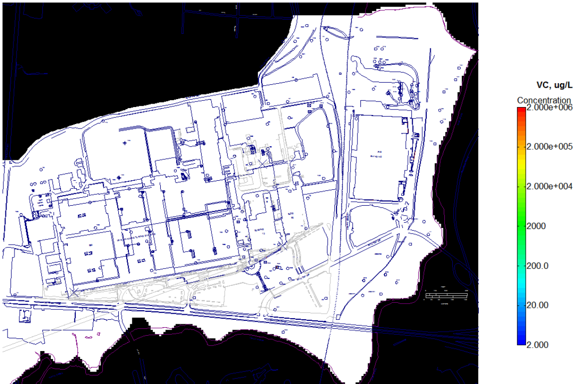
Future Conditions: VC, Year 93, 30 years after complete source dilution Future Conditions, 0% Source Concentration Reduction, 75% Source Duration Reduction
