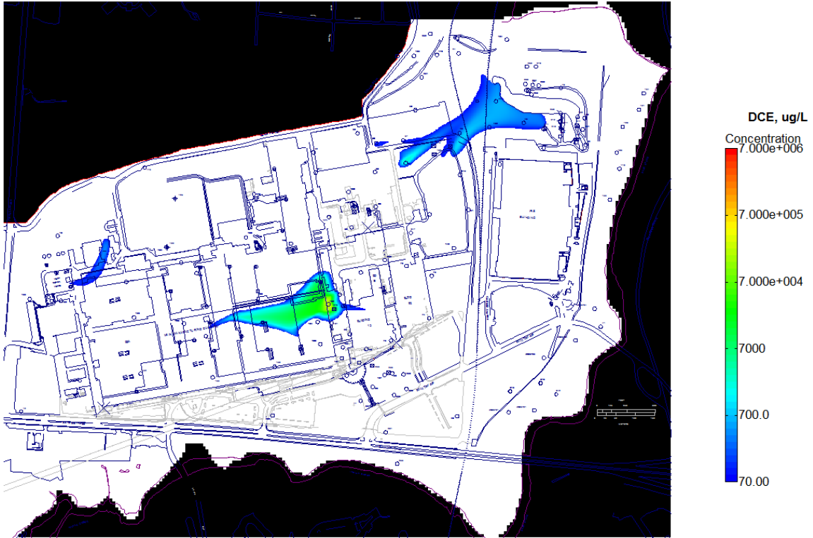
Current Conditions: DCE, 31 TO 63, source concentration stable
