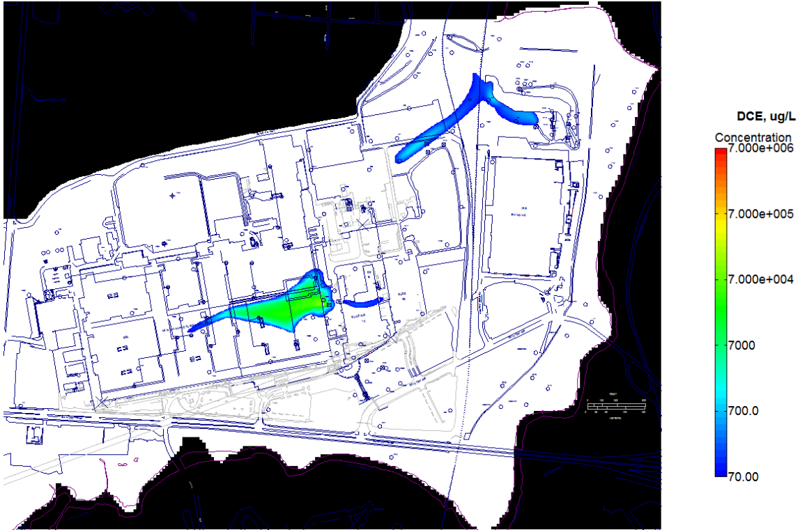
Current Conditions: DCE, Year 255, 5 years after complete source dilution
