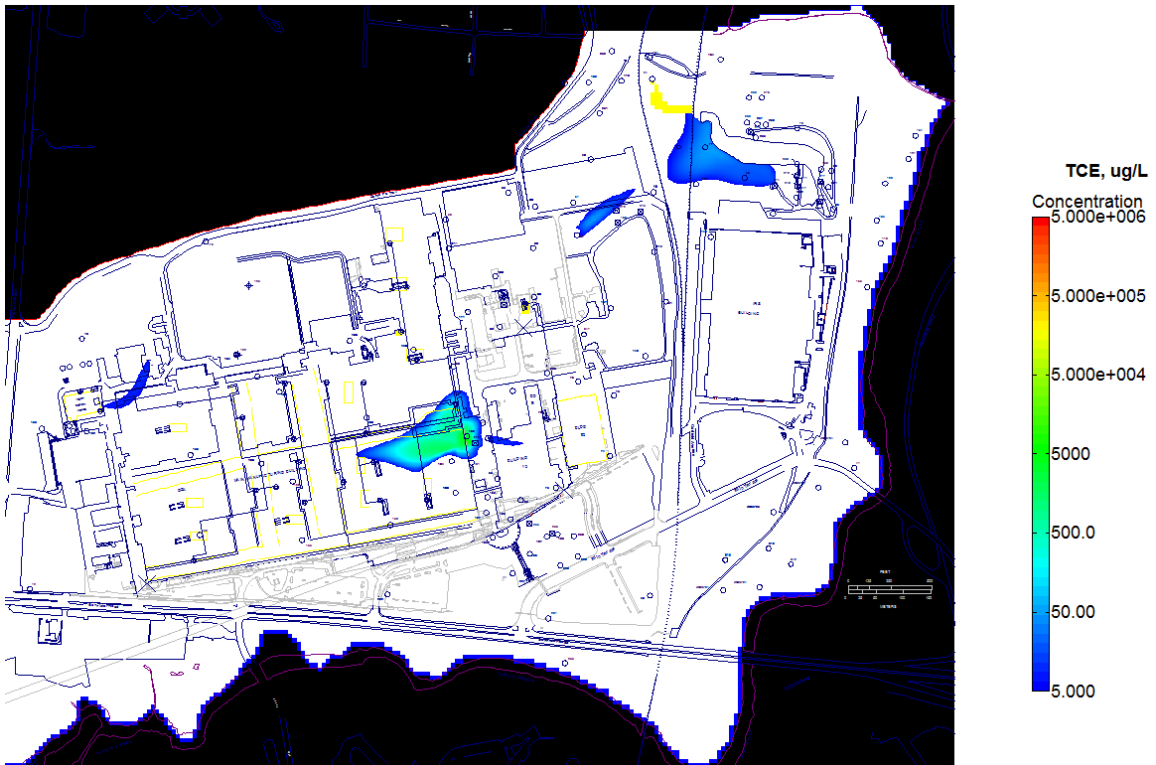
Current Conditions: TCE, Year 128, 128 year after source remediation
