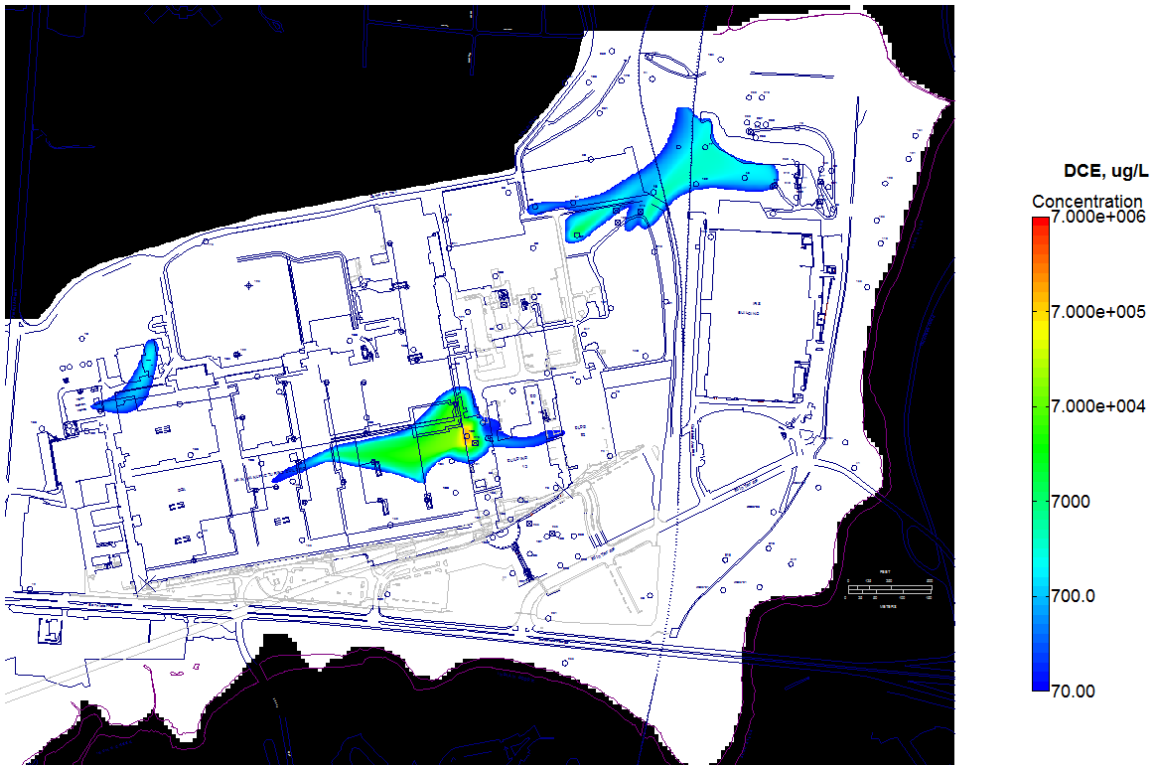
Current Conditions: DCE, Years 1 through 250, constant source Current Conditions, No Source Reduction
