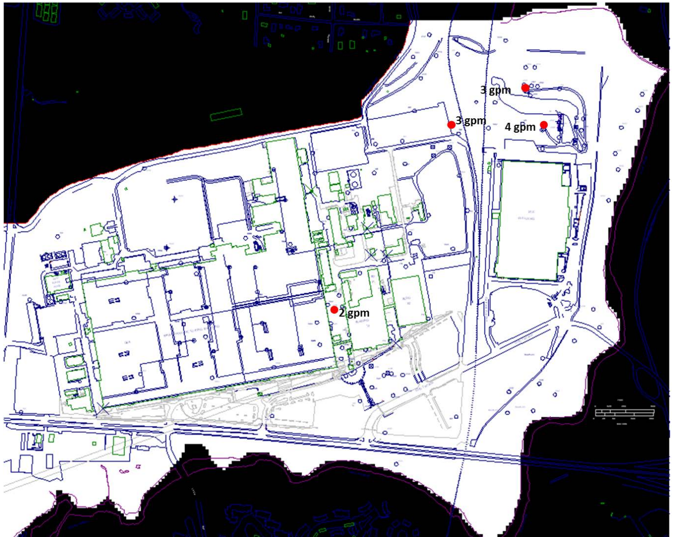
Figure 75. Current condition extraction well locations.
